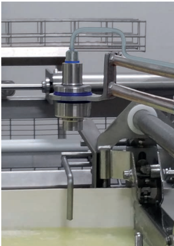
Level measurement in cheese production
